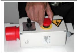
3. Check that the emergency stop button is in the out position. If not rotate it clockwise to recease.
