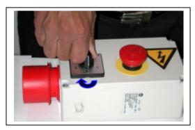
2. Turn the motor switch to the "OFF" position.
